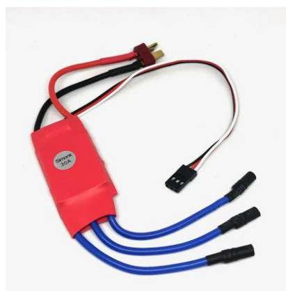
Figure 3: Simonk 30A ESC (Electronic Speed Controller)
